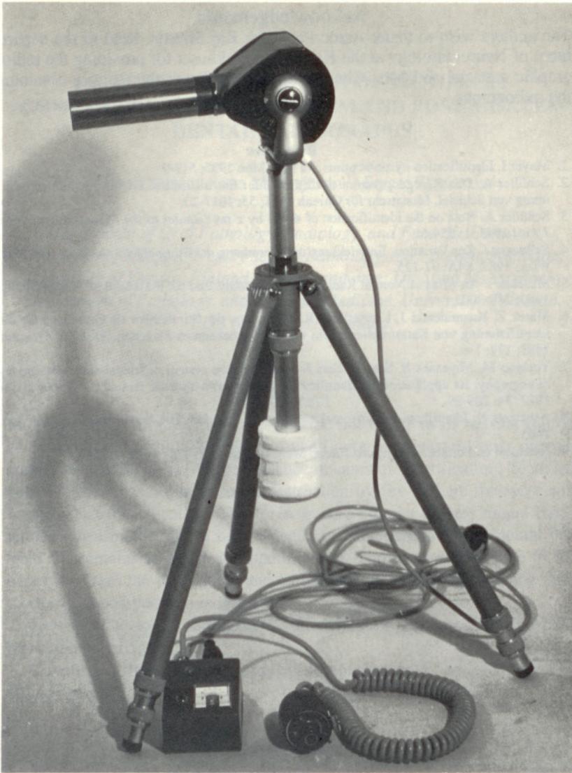
Fig. 6 An example of a portable dental radiographic unit which can be used to radiograph the sinus frontalis.
