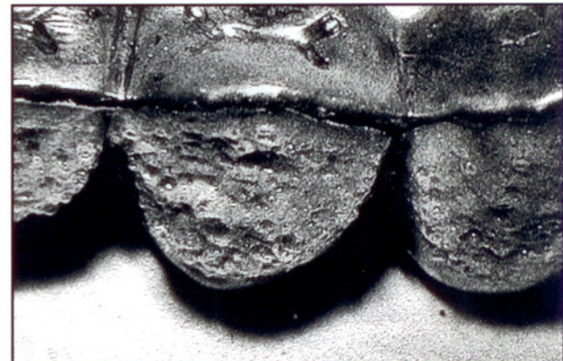
Fig.6: Stereomicroscopic image (20X) of a bridge covered with acrylic resin after exposure to 400°C. There is partial degradation and loss facing material. The alloy shows the first signs of oxidation with discolouration
