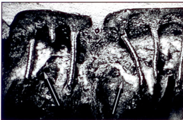
Fig.7: Stereomicroscopic image (8X) of a bridge covered with acrylic resin after exposure to 600°C. The loss of the facing can be seen while traces of the bonding system used at the alloy-facing material (silane) interface can be found on the surface of the alloy which has remained intact
