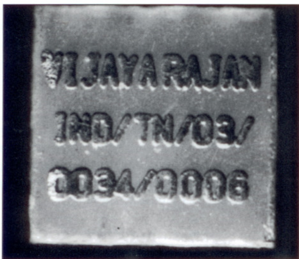
Fig.1: Denture-marking microchip with inscription. Dimensions 5mm x 5mm x 0.6mm
