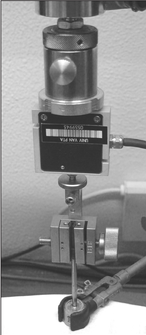
Fig 1: The specially designed metal plunger in the Zwick Z1010 compression tester.
