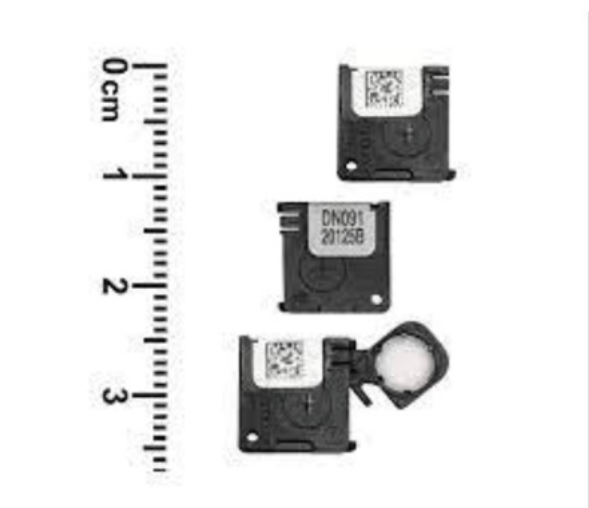
Figure 2. The NanoDot™ Optically Stimulated Luminescence (OSL) Dosimeters (Landauer, IL, USA) modified into a ring using ring binder.
