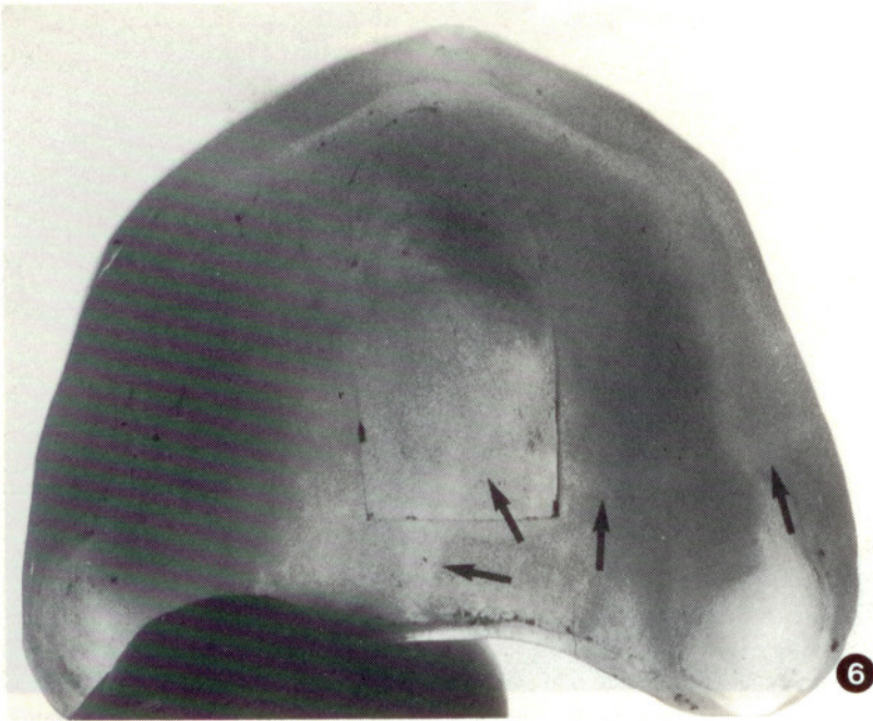
Fig. 6. The L-shaped repair-like mark (arrowed) which was not a repair.
