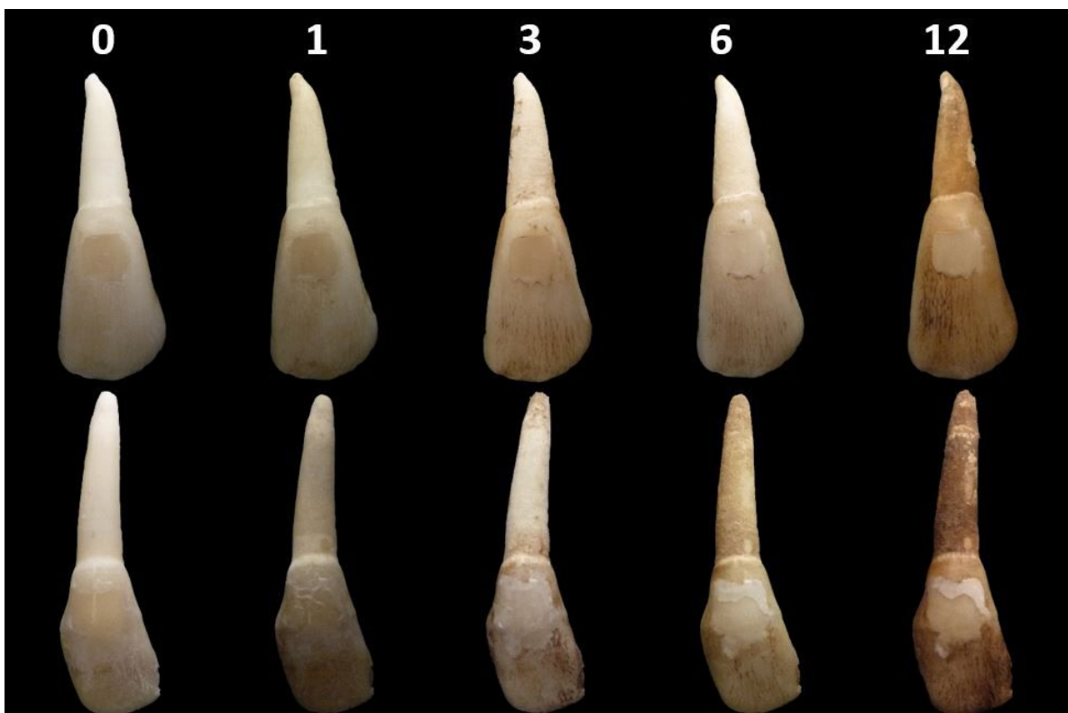
Figure 6: A photographic comparison of the restorations of CR (above) and GIC (below) submitted to different periods of submersion in water.
