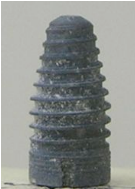
Fig.3. The Nobel Biocare Replace Select™ 4.3 x 8mm after incineration.
