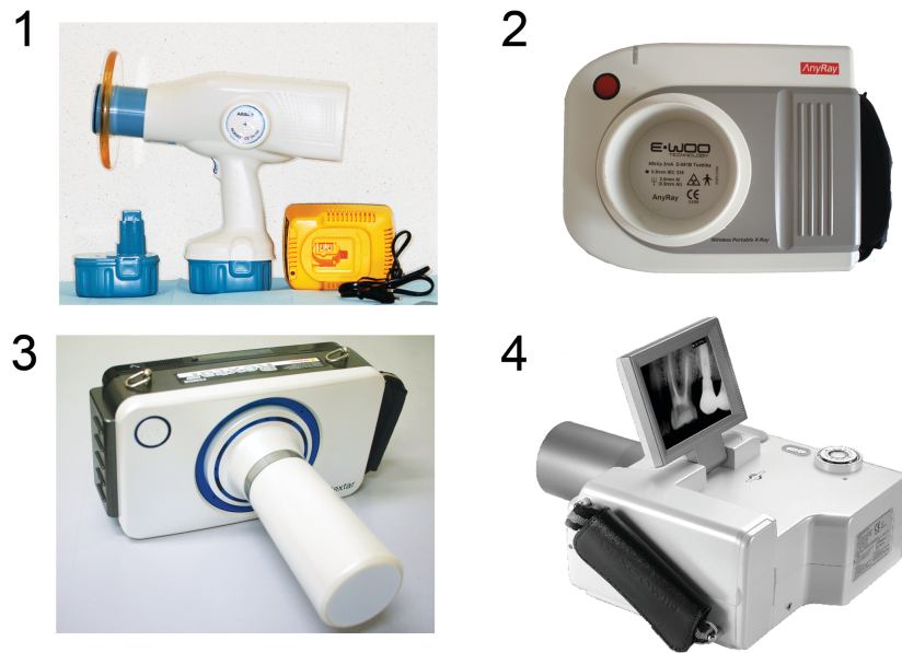
Fig. 4: Several portable dental x-ray devices are available on the market nowadays. (1) Nomad ® (Aribex, Utah, USA) was first introduced in 2005 in the identification process after Tsunami disaster. (2) AnyRay ® (VATECH Co., Ltd., Gyeonggi-do, Republic of Korea), (3) Rextar ® (Sungwon Econet, Seoul, Republic of Korea) (4) ADX4000 (DEXCOWIN Co., Ltd. Seoul, Republic of Korea)
