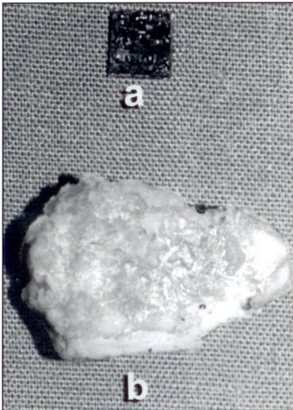
Fig. 3: Microchip embedded in acrylic resin blocks ( a ) after heating at 600°C, ( b ) after immersion in sulphuric acid at eight weeks
