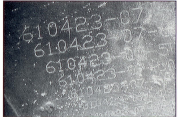
Fig.6: The sample ID marking of varying, decreasing size made on a cobalt-chromium test plate, seen under a stereo-microscope. The height of the characters in the third row is estimated to be 250 \mu\text{m} at 20X magnification
