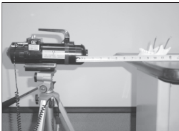
Fig.1: XR-150™ portable x-ray unit mounted on a tripod
