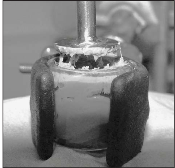
Fig 2: The retraction of the plunger in a “sticky” Impregum sample is demonstrated at 120 days.
